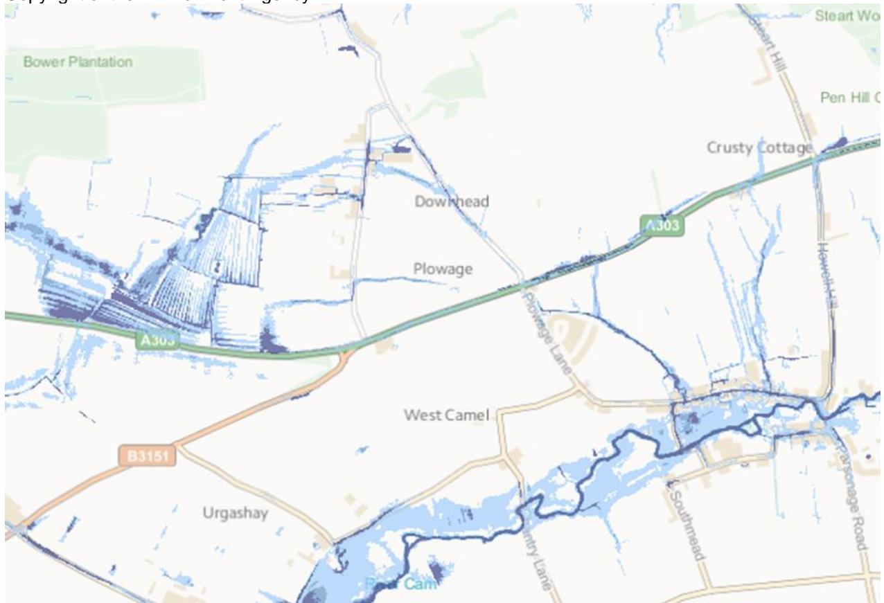
Figure 4.4 The Environment Agency surface water flood risk map showing flooding on the existing A303. Copyright of the Environment Agency.
